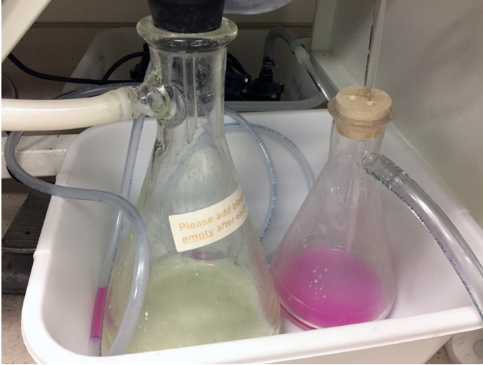
Contaminated vacuum flask and tubing (seen in the second vacuum flask containing pink media).
